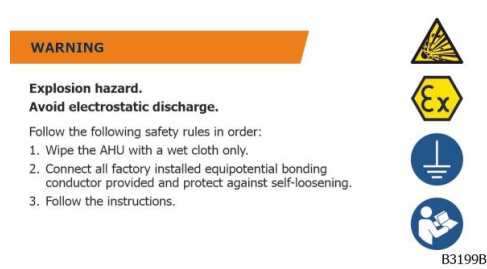
Fig. 7: Warning sign: "risk of explosion from electrostatic discharge"
