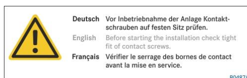
Fig. 4: Warning sign "Check contact screws"
