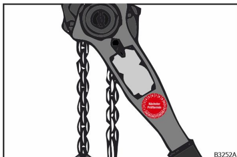
Fig. 105: inspection sticker (lever chain hoist)
